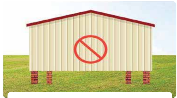
NO INSTALLS ON STACKED BLOCKS
