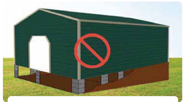
NO INSTALLS ON UNEVEL LAND
