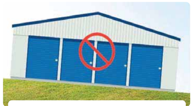
NO INSTALLS ON SLOPES OVER 12"
