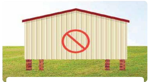
NO INSTALLS ON STACKED BLOCKS
